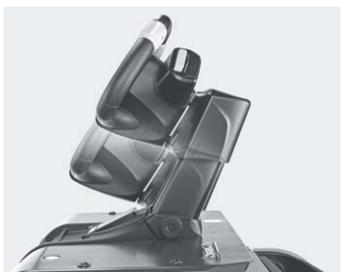
Maximum ergonomics due to the height-adjustable steering wheel and improved angle for individual driver preferences
